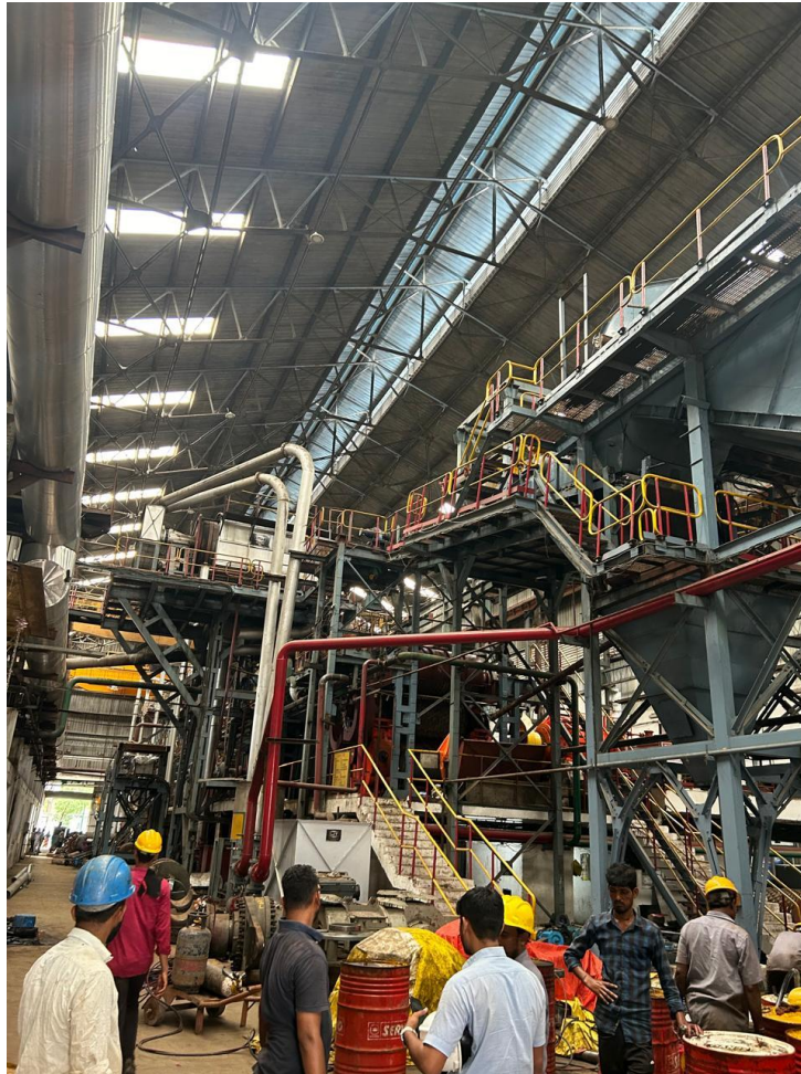
Picture 3: (a) Mill house where the cane is crushed to extract juice and (b) Centrifugal section used for separation of sugar crystals from the molasses
