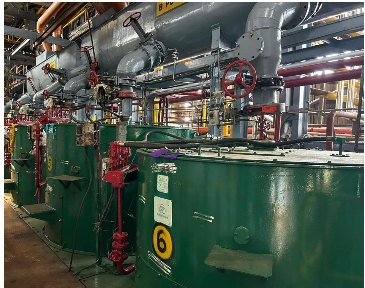
Picture 3: (a) Mill house where the cane is crushed to extract juice and (b) Centrifugal section used for separation of sugar crystals from the molasses
