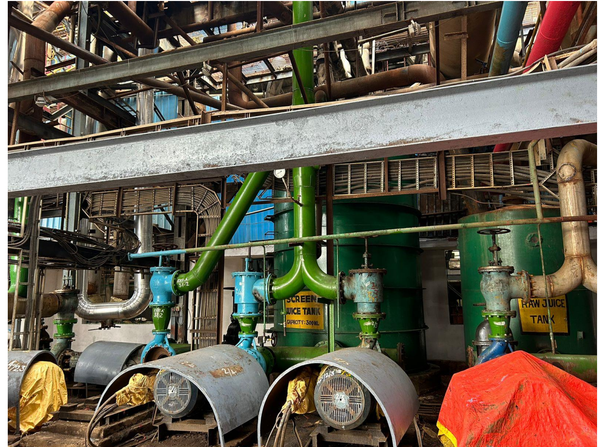
Picture 2: Boiling house where impurities are removed from sugarcane juice
